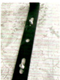
2. Drill 2 holes with an M10 drill bit on the surface according to the two marks.
