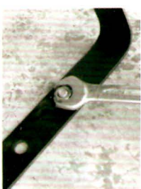
7. Tighten the two nuts with wrench.
